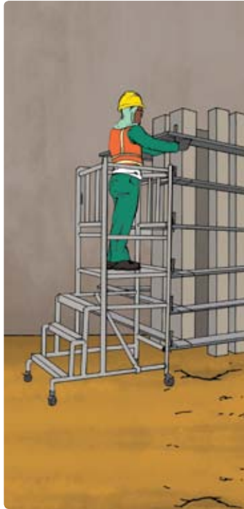
Formwork is erected from below using podium steps
