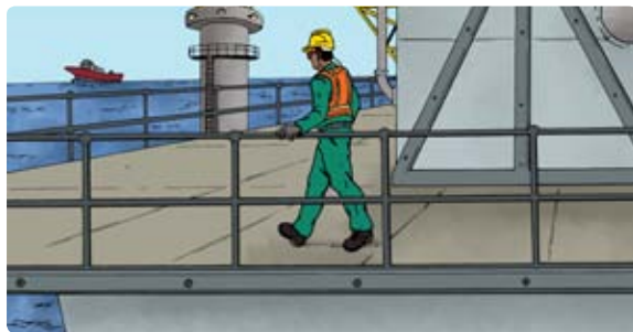
Permanent edge protection on frequently accessed area on oil rig
