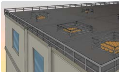
Roof openings have a different type of protective measure
