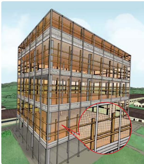
Advanced protection (used in high-rise construction) – full-height perimeter screens
