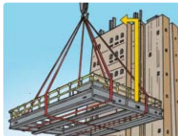
Install guardrails before erecting a structure
